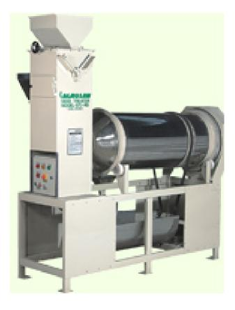
Slurry tanks have 15 to 35 gallon capacities, depending upon the size of the treater. They are equipped with agitators that mix the slurry in the tank and keep it suspended during operation. It is important that the powder be thoroughly suspended in water before treating. If the treater has been idle for any period of time, sediment in the bottom of the slurry cups must be cleaned out.
